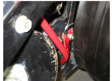
**General Mounting Instructions:** Your SmartBox® system requires that a minimum 45 degree angle be maintained at any point along the product discharge path from the meter outlet to the in-furrow drop tube. The drop tube may need to be bent to adjust. The plastic hose should be cut to length to eliminate any unnecessary slack that could cause a flow restriction. Also, if using a seed firmer the drop tube's foot (if applicable) may need to be cut off or bent up if restricting the firmer's travel.
